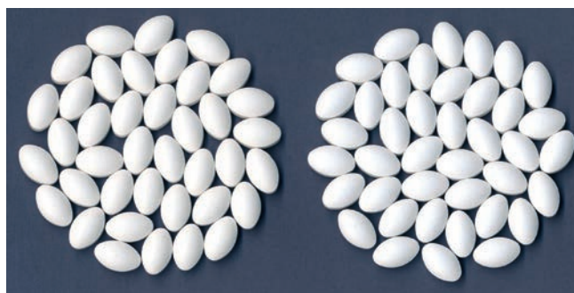
Left: SheffCoat™ TF, applied as a 15% dispersion in water to a 6% weight gain at a tablet bed temperature of 42-44°C
